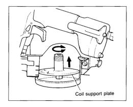
Place the nail coil over the coil support plate. Uncoil enough nails to reach the feed claw. Place the first nail in the driver channel and the second nail in the feed claw. The nail heads must be in the slot in the feeder body. Place other uncoiled nails on feeder body. Close the magazine cap and door after checking to see that the nail coil is set properly in the magazine.
